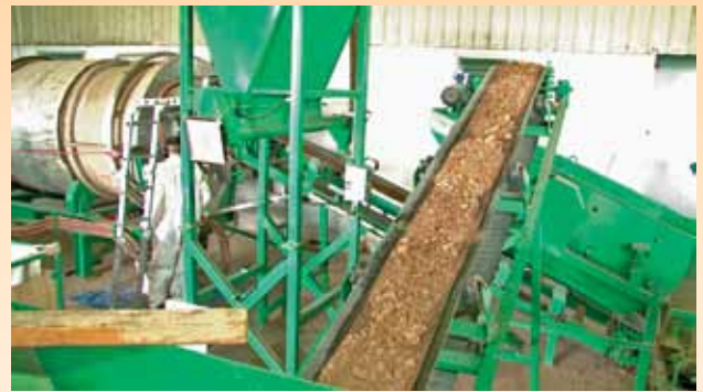
Contaminated soil heading to the dryer
